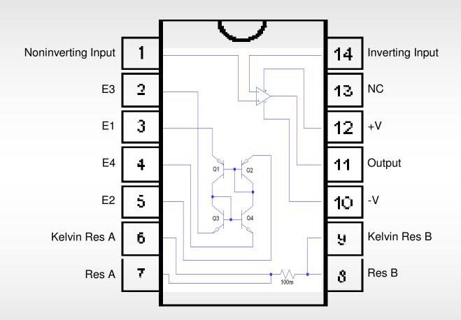
Q1 thru Q4 are lot-matched and thermally-bound high voltage transistors. They are interconnected to form a current mirror which allows the user to sense the current in either a high positive or high negative volt power supply line, for use up to 300 Volts. The internal precision 100 milliohm current sense resistor is connected in series with the line, and Kelvin connections to the resistor provide the most accurate sensing of the voltage drop.
